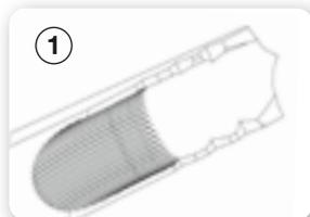
1 The bilow-grind claws radially into the teeth and avoids a "riding" in-between the tooth crown and the inner contour of the beak.
