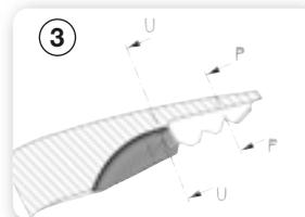
3 The different deeply elaborated inner contours ensure maximal adaptation on the teeth in different actualities. No tilting of the teeth while rotary and/or lifting movement.
